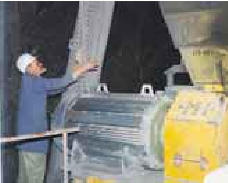
*Electrical Engineer Walter Büchel on the 355 kW motor of the biggest rotary crusher that reduces 5,000 tons of stone a day. With the old time-controlled Y/delta switching system, varying charges of stone and fluctuating temperature caused problems with high starting currents. Y/delta starting in the case of the new electronic control and protection system of the 825 series is current-controlled and therefore always takes place at the right instant for minimum current.*
