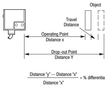
The high hysteresis in most photoelectric sensors is useful for detecting large opaque objects in retroreflective, polarized retroreflective and transmitted beam applications. In diffuse applications a large difference in reflected light from target and background also allows the use of high hysteresis sensors.
