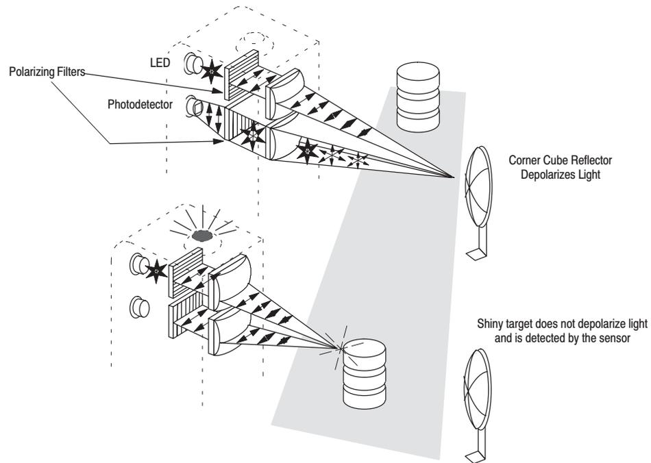
Polarized retroreflective sensors offer 30%–40% shorter range (and less margin) than standard retroreflective sensors. Instead of infrared LEDs, polarized retroreflective sensors must use a less efficient visible light source (typically a visible red LED). There are additional light losses caused by the polarizing filters.
