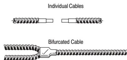
Two individual cables are used for transmitted beam sensing. Some individual cables are packaged separately, others are sold in packages of two. Order carefully to receive two cables.
