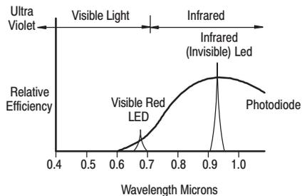
The invisible (infrared) LED is a spectral match for this silicon phototransistor, and has much greater efficiency than a visible (red) LED.
