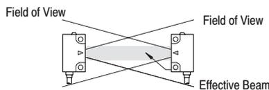
Detection of objects smaller than the effective beam can best be achieved by reducing the beam diameter through means of apertures placed in front of the light source and receiver (Figure 7). Apertures are available for most 42KL, 42KB and 42EF transmitted beam sensors. Some users have created their own apertures for other sensor families.
