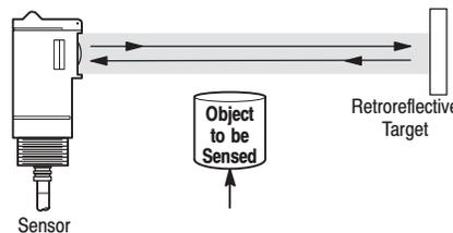
Special reflectors or reflective tapes are used for retroreflective sensing. Unlike mirrors or other flat reflective surfaces, these reflective objects do not have to be aligned perfectly perpendicular to the sensor. Misalignment of a reflector or reflective tape of up to 15° will typically not significantly reduce the margin of the sensing system (see Figure 9).
