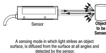
There are a number of different types of diffuse sensing. The simplest, *standard diffuse*, is discussed here. Other types, sharp cutoff diffuse, fixed focus
