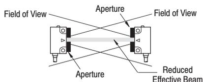
The most reliable transmitted beam applications have a very high margin when the target is absent, and a margin of zero (or close to zero) when the target is present.
