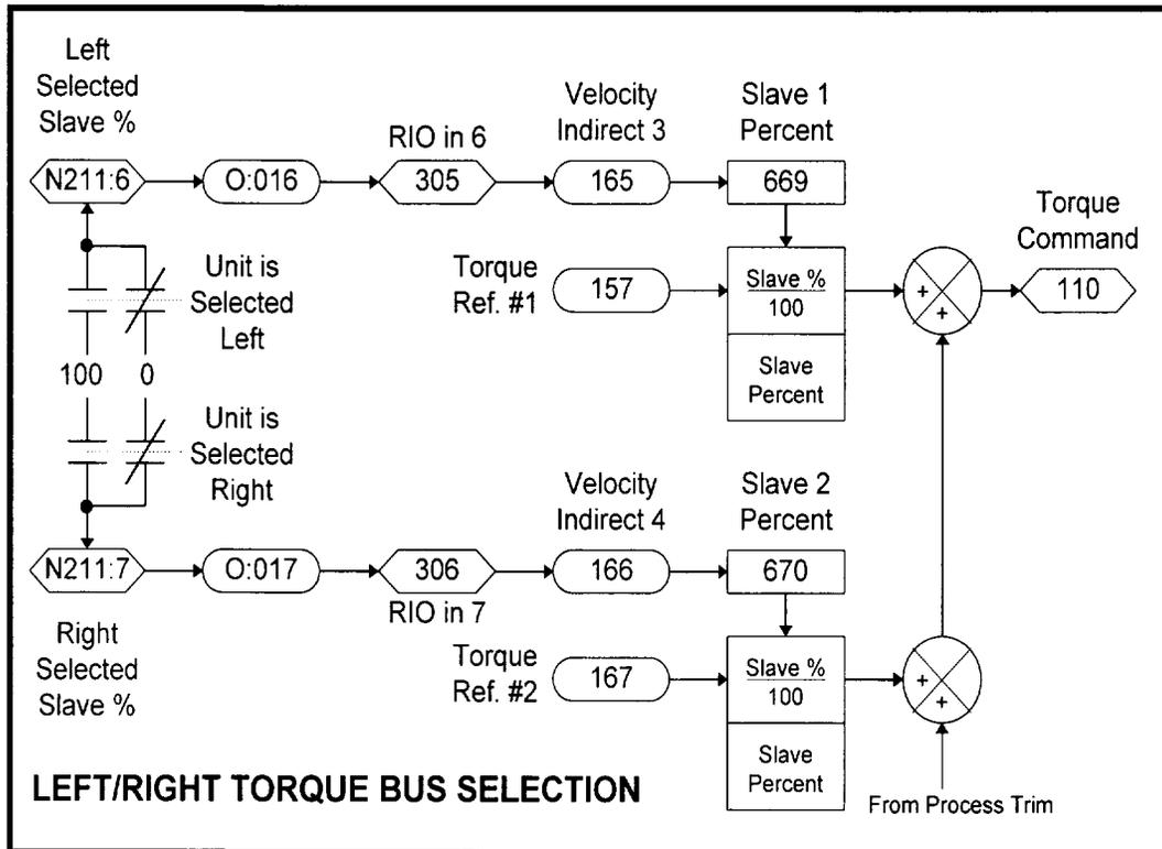
During the tuning process, it will be necessary to select the right/left selectable units in both directions and adjust the appropriate analog zero and scale parameters.
