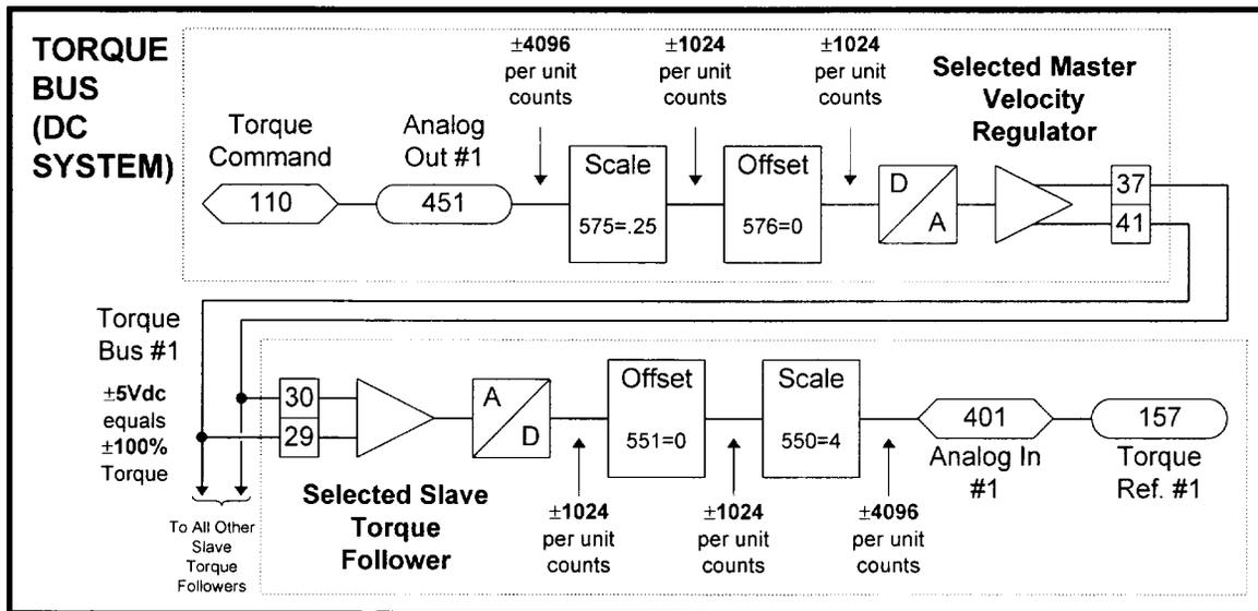
The diagram above illustrates the analog signal path for only one torque bus. If the system contains selectable master velocity regulators, a second torque bus will exist. The second torque bus will enter the slave torque follower through the second analog input which will be scaled and offset in an identical manner to the first analog input. The second analog input, drive parameter 402, will be linked to drive parameter 167, Slave Percent 2.
