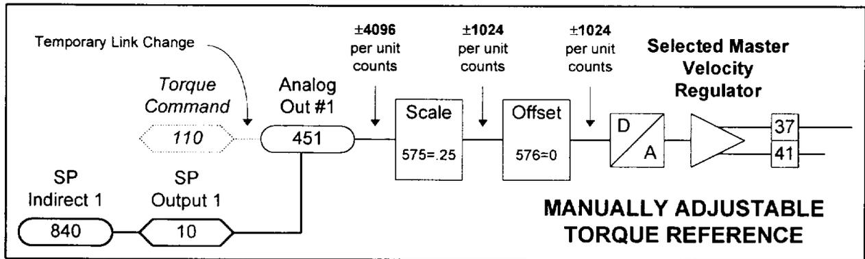
6. Connect a DMM to terminals 37 and 41 of TB3 on the Master Drive.
