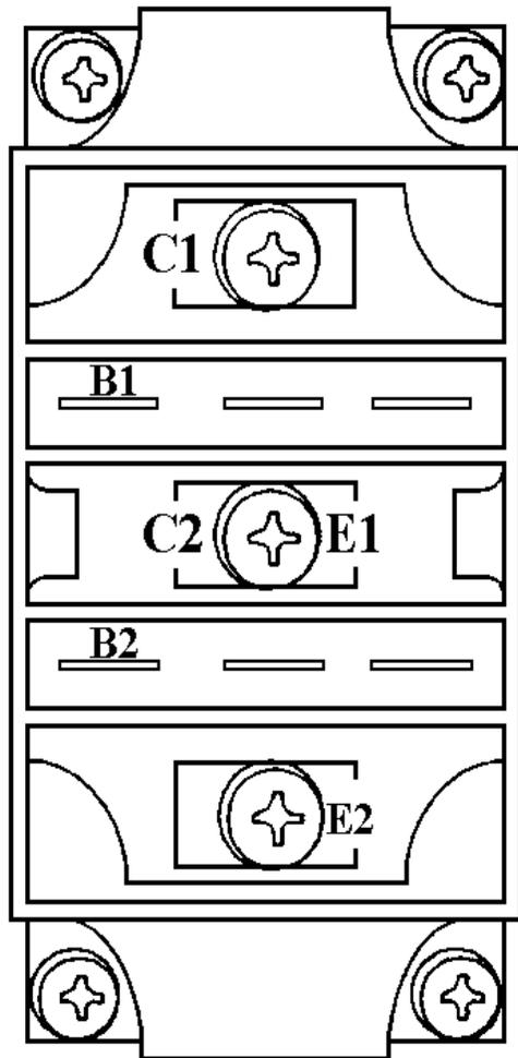
With an ohmmeter set on the x1 scale, measure the resistance between the collector and emitter of each module as follows.
