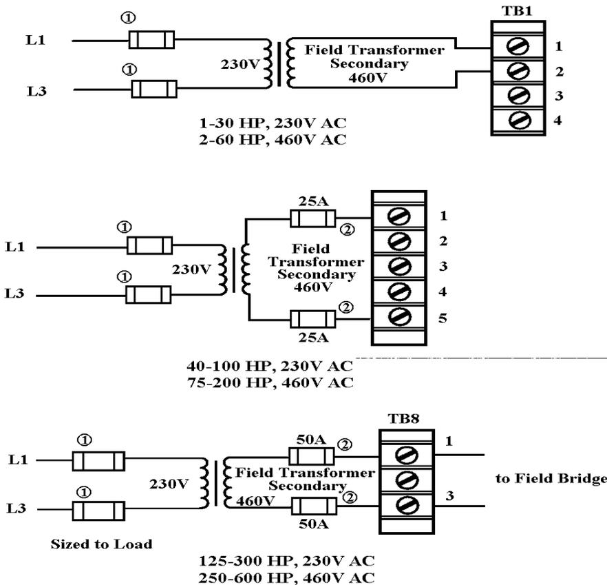
1. The primary of the external field transformer requires branch circuit protection, to be fused with FRN or FRS style fuses. Refer to NEC Code (and local codes) for sizing.
