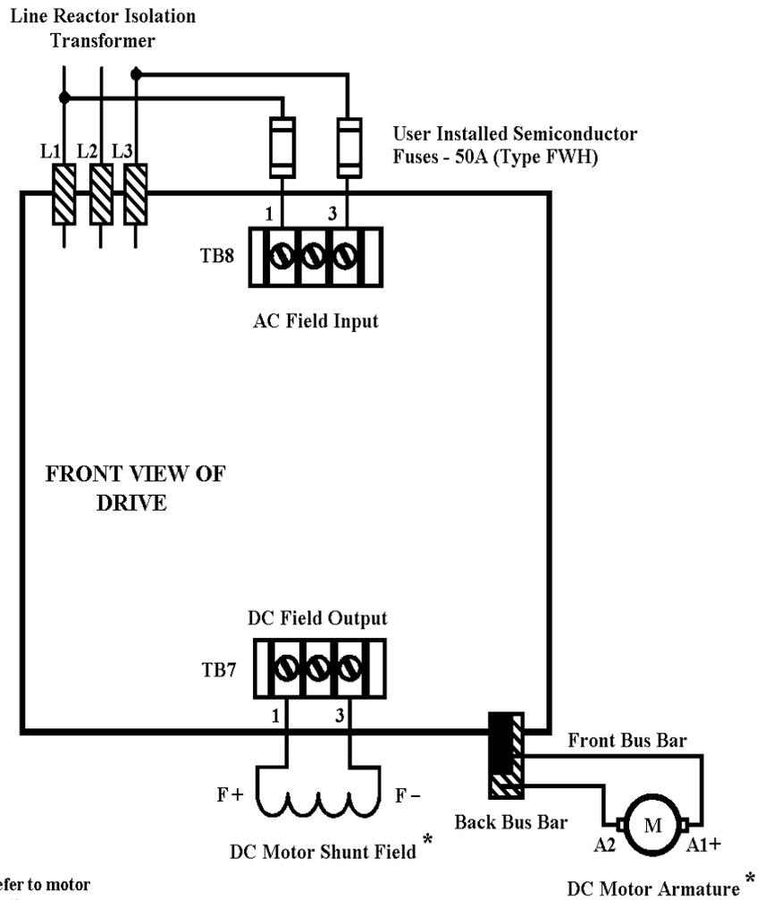
\* Typical motor connection. Refer to motor data for specific motor connections.
