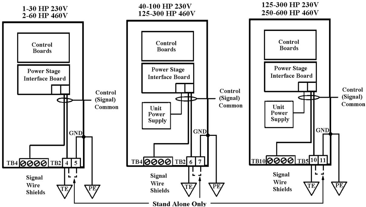
**Signal Ground (TE)**- The Signal Ground point is used for all control signals internal to the drive. Depending on the application, TE may be connected to a system TE bus or connected to PE ground. Figure 6 and 7 illustrate the possible connections for TE. If the drive is configured as a **stand alone unit**, the TE and PE grounds may be run individually to the drive, or a jumper can be placed as shown in Table C and one ground lead run as indicated in Table D.
