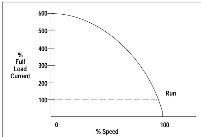
In addition to high starting currents, the motor also produces starting torques that are higher than full load torque. The magnitude of the starting torque depends on the motor design. NEMA publishes standards for torques and currents for motor manufacturers to follow. Typically, a NEMA Design B motor has a locked rotor or starting torque that is about 180% of full load torque.
