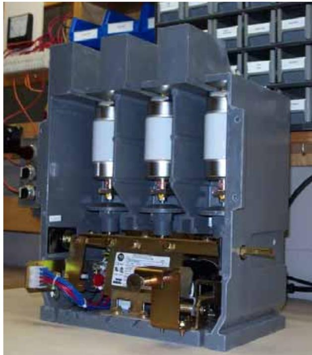
Figure 11 – Complete Contactor after Conversion
