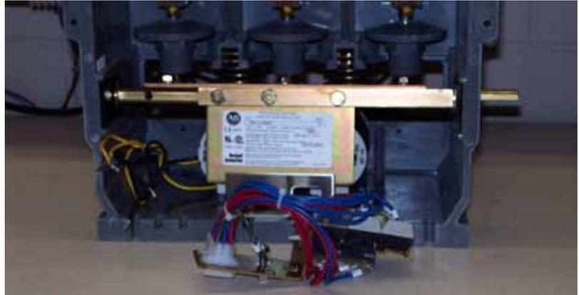
Figure 3 – Disconnecting Coil Leads from Auxiliary Contact Assembly
