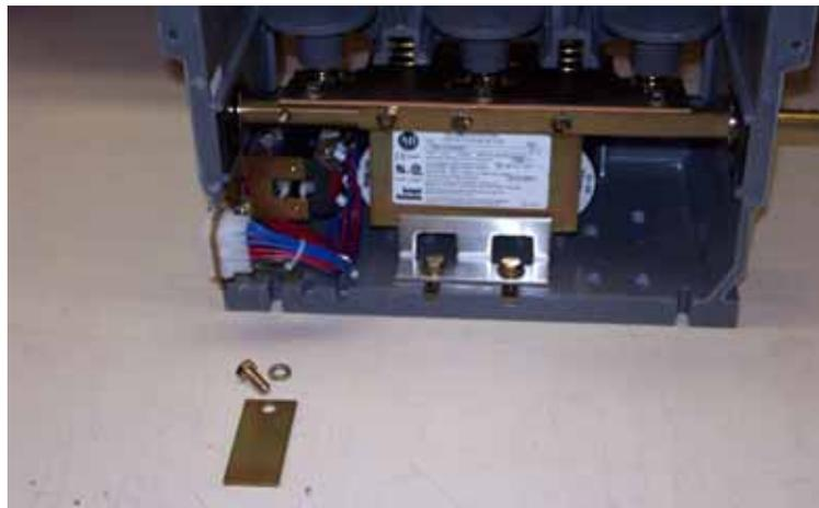
Figure 3 – Removing the Auxiliary Contact Actuator Plate
