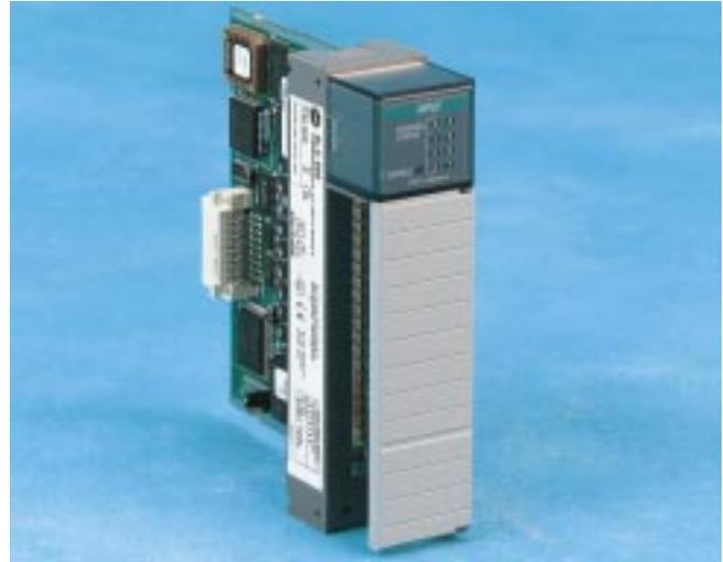
The new 1746-NR8 RTD module offers advanced performance features for temperature measurement and control applications with large numbers of RTD or resistance inputs. This module has excellent accuracy and compatibility with various RTD types (e.g. platinum, nickel, copper, nickel-iron) or other resistance inputs and supports connections from two or three wire RTD sensors.
