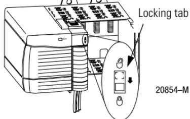
3. To lock the RTB on the module, slide the locking tab down.
