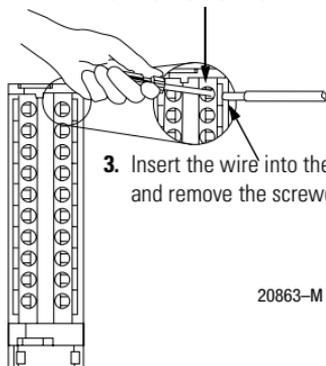
3. Insert the wire into the open terminal and remove the screwdriver.
