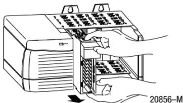
2. Pull module out of the chassis.
