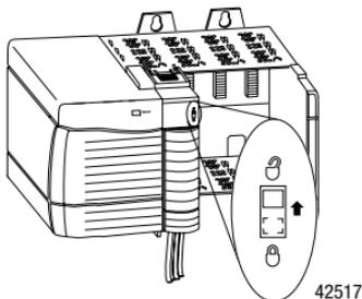
2. Open the RTB door and pull the RTB off the module.
