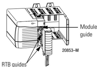
2. Press quickly and evenly to seat the RTB until the latches snap into place.
