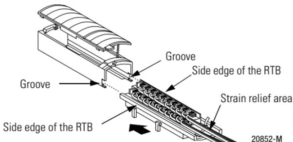
2. Slide the RTB into the housing until it snaps into place.
