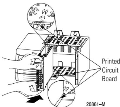
2. Slide the module into the chassis until the module locking tabs click.
