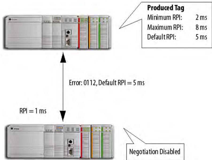
**Version 17 and earlier:** The RPI requested by the consumed tag is not within the range of the producer. The connection is rejected and a 0112 error is reported that the connection failed. You must re-enter an RPI that is within the range configured on the produced tag. If a version 17 consumer is trying to connect with a version 18 producer and the RPI is outside the range of the producer, a 0112 error reports the connection failed.
