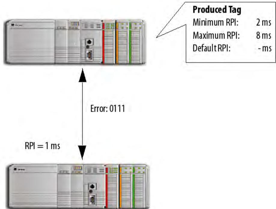
**Version 17 and earlier:** The RPI requested by the consumed tag is not within the range of the producer. The connection is rejected and a 0111 error is reported that the connection failed. You must re-enter an RPI that is within the range configured on the produced tag. If a version 17 consumer is trying to connect with a version 18 producer and the RPI is outside the range of the producer and there is no default set up, a 0111 error reports the connection failed.
