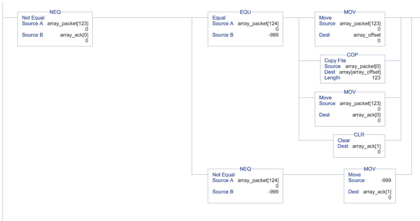
Transferring a large array as smaller packets improves system performance over other methods of transferring the data.
