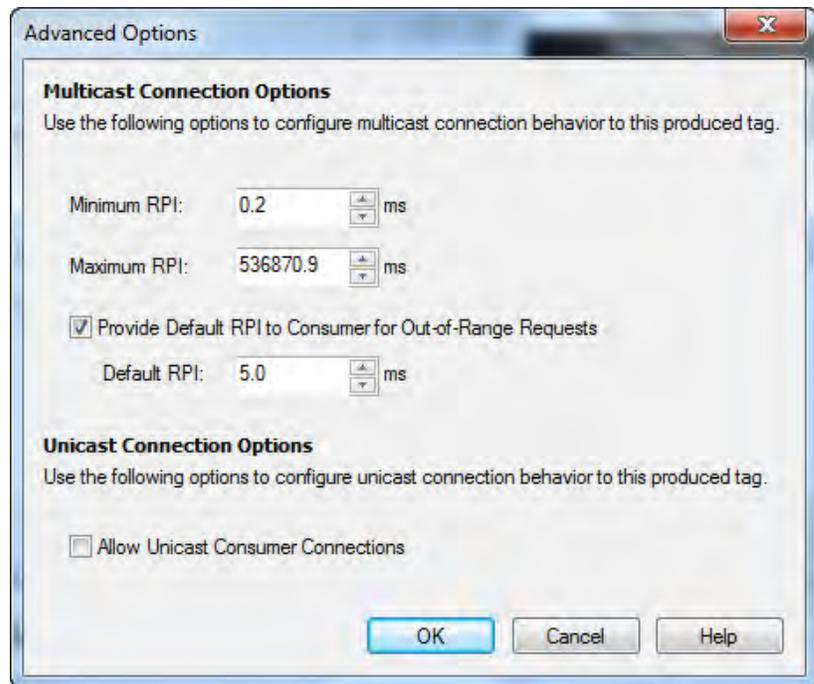
**Important:** A unicast connection between a consumer and producer controller is the default on the **Advanced Options** dialog check box. Multicast connections can be changed to a produced tag whether or not the box is checked. The check box dictates only whether this produced tag can accept a unicast connection. The consuming controller determines if the connection is unicast.
