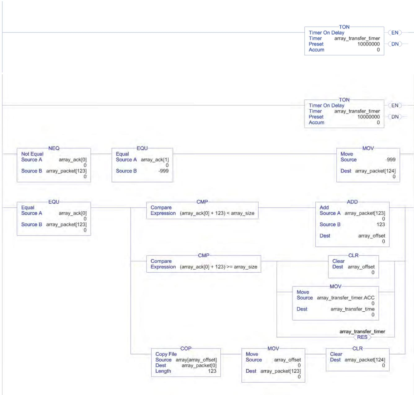
If the current transfer time is greater than the maximum transfer time, update the maximum transfer time. This maintains a record of the longest time to transfer data.
