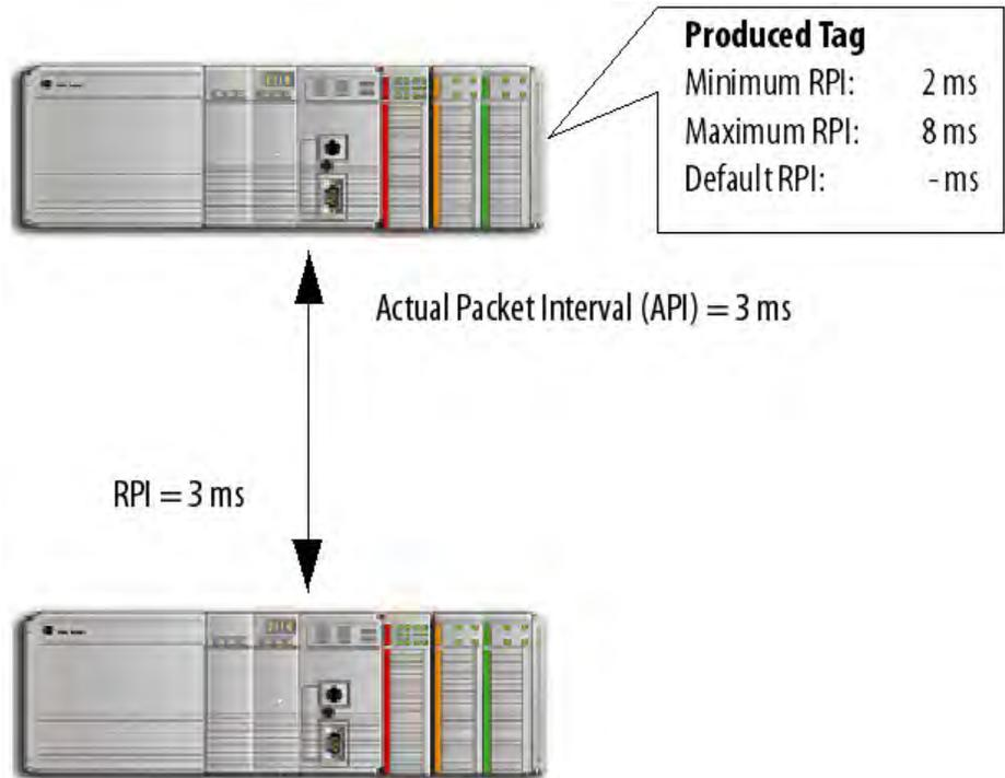
**Version 17 and earlier:** The consuming controller is brought online with an RPI configured at 3 ms. The producer accepts the RPI requested by the consuming tag. All controllers on the multicast connection will be increased to 3 ms for the API, which is the interval the data is actually being produced.
