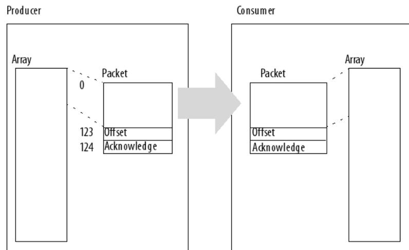
In addition, the array must contain an extra 122 elements. In other words, it must be 122 elements greater than the greatest number of elements that you want to transfer.
