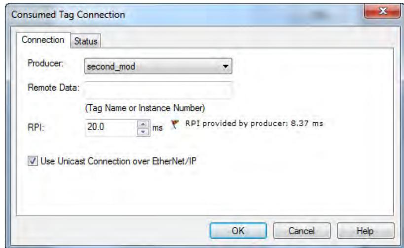
The RPI that had been requested by the consuming controller is dimmed. This lets you view the time interval the consuming controller had requested and the RPI provided by the producing controller.
