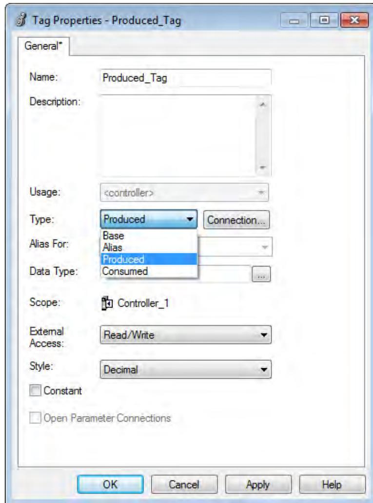
4. In the **Tag Properties** dialog box, in the **Name** box, type the name of the produced tag.
