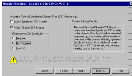
The CST does not start in this chassis until a connection is made with the CST master, typically at module power-up. If there is no connection to the CST master at power-up, the module faults and has no CST until the connection is made. This is for **firmware revision 2.10 only**. To see how this works with firmware revision 2.18 or greater, see page 4.
