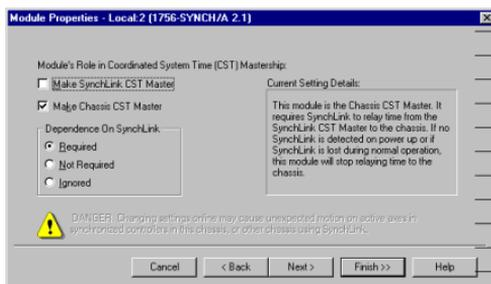
The previous module revision (i.e. 1.17) only offered this option when communications with the CST master are lost.
