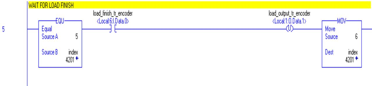
**Rung 5:** When the handshake input from the encoder (load finish) is set, clear the strobe output.
