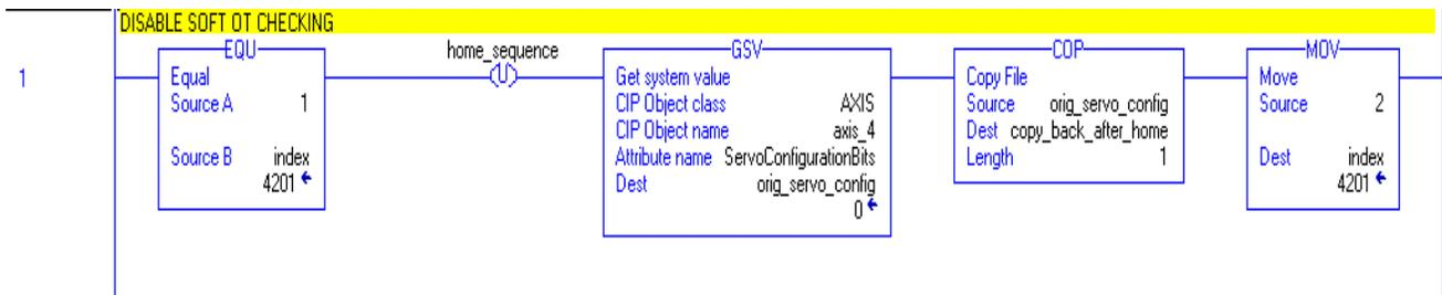
**Rung 1:** Clear the home\_sequence bit and get the servo configuration. This is later used to determine if the axis has software overtravel enabled or not. When you get this value, copy it to another tag so that it can be replaced at the end of the checking procedure.
