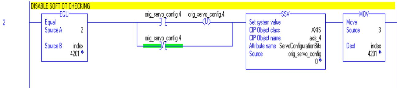
**Rung 2:** Check to see if the ‘Soft Over Travel Checking’ is enabled. If it is, turn it off and save the value to the servo module.
