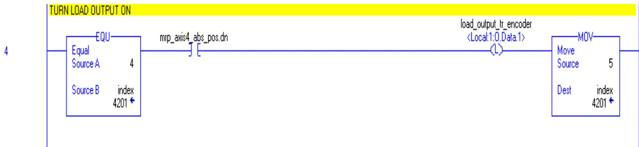
**Rung 4:** When the redefine is completed, set the strobe output (or load output) to the encoder.
