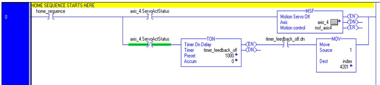
**Rung 0:** When home\_sequence is set, check to see if the feedback is on. If it is, turn it off and wait for the axis to come to a stop.
