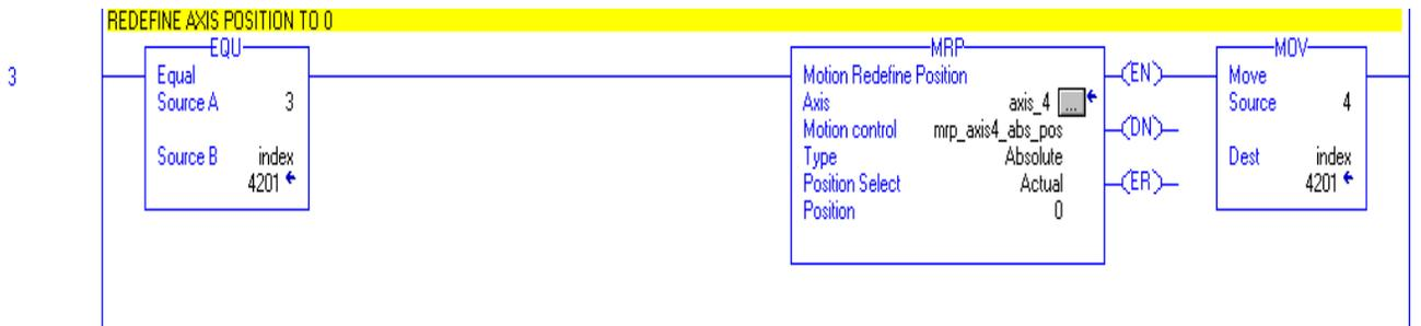
**Rung 3:** Clear the Actual\_Position Accumulator so the value from the encoder can be stored in it.
