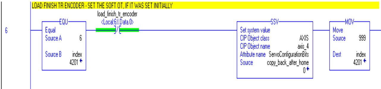
**Rung 6:** When the handshake input gets cleared from the encoder, the position data is sent to the controller, and the actual\_position is received from the encoder. The Software Over Travel checking can be restored, if it was enabled by saving the original value to the Servo Module.
