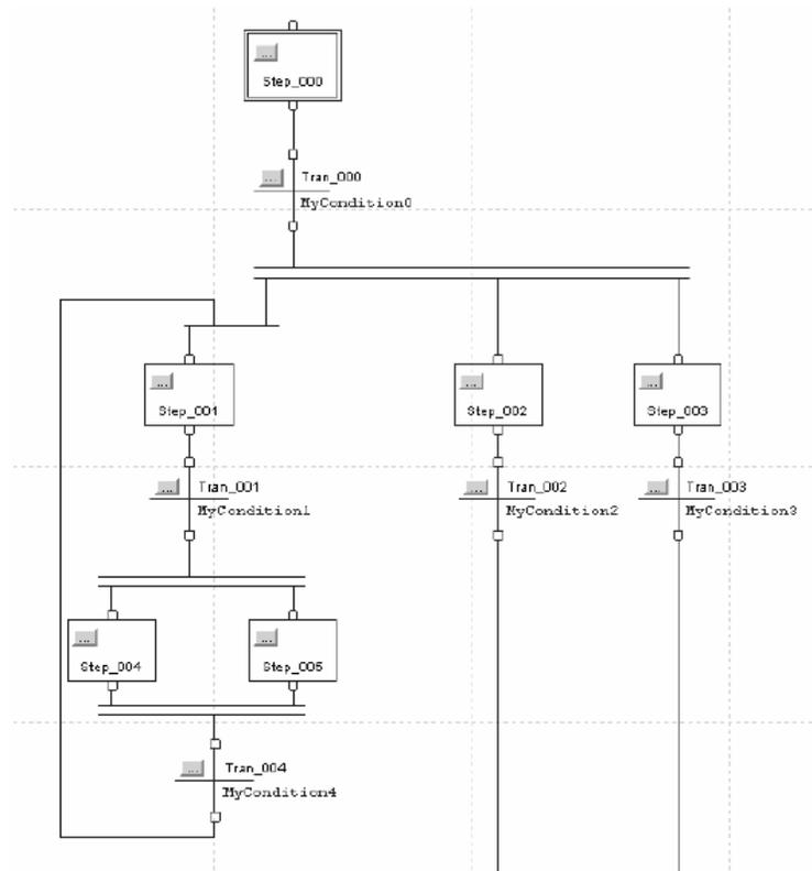
Execution starts at Step\_000. When Tran\_000 becomes true, Step\_001, Step\_002 and Step\_003 should become active. However, because the nested simultaneous branch in the left path converged and looped back to its parent step (Step\_001), the active steps were actually **Step\_005**, Step\_002 and Step\_003.
