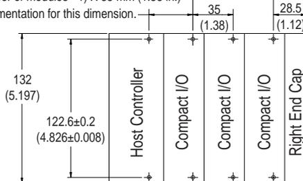
NOTE: All dimensions are in mm (inches). Hole spacing tolerance:  $\pm 0.4$  mm (0.016 in.)
