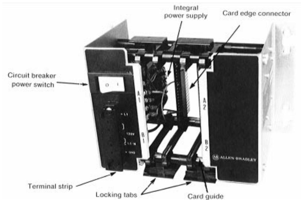
The two-slot chassis assembly (figure 1) consists of:
