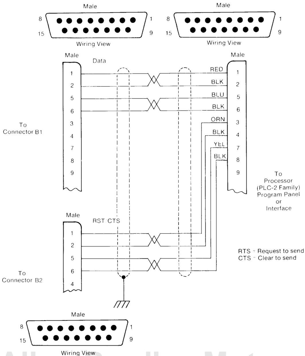
**Step 5** – Connect the industrial terminal Channel A PLC-2 family connector to the two line drivers B (female) connectors using a 1770-CW2 interconnect cable. Attach cables so that stress is relieved at the connector hoods. Refer to figure 8.
