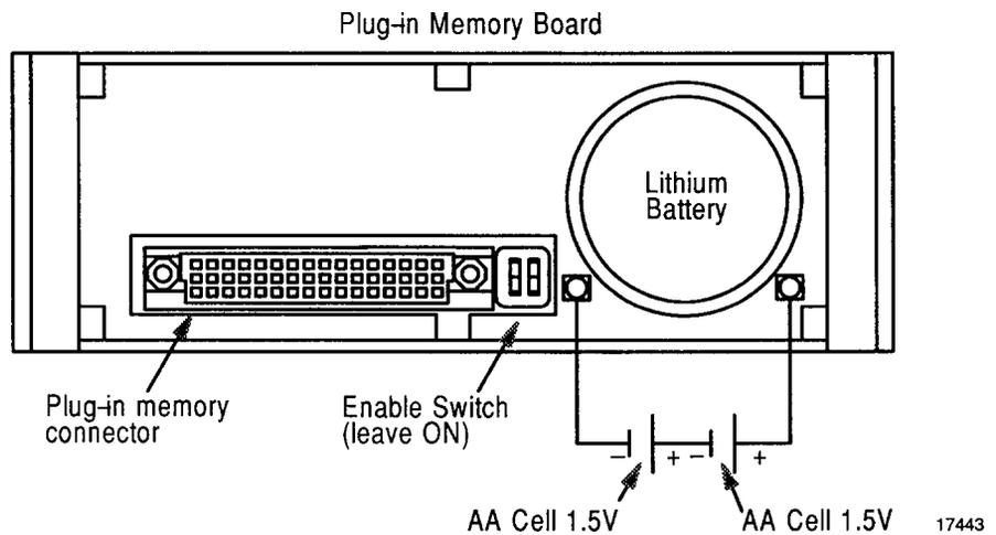
6. Connect external batteries to the supplied test points on the memory board.
