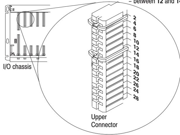
You can change the position of these bands if subsequent system design and rewiring makes insertion of a different type of module necessary.
