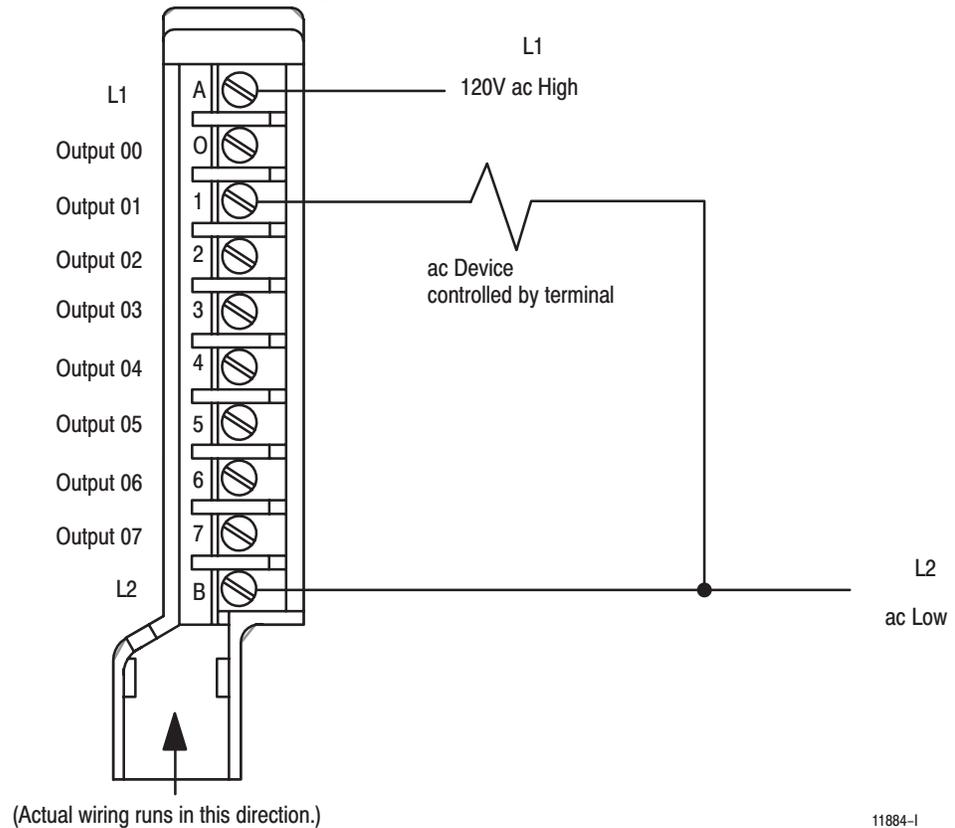
You can use an output of the 1771-OA module to drive an input of a 120V AC input module (1771-IA, -IA2, -ID and -IAD) to indicate status, such as the turning on a motor starter (Figure 2). However, you must add an external resistor between the output terminal and the common (L2) (Figure 2). Typically, this is a 2.5K ohm, 10W resistor.
