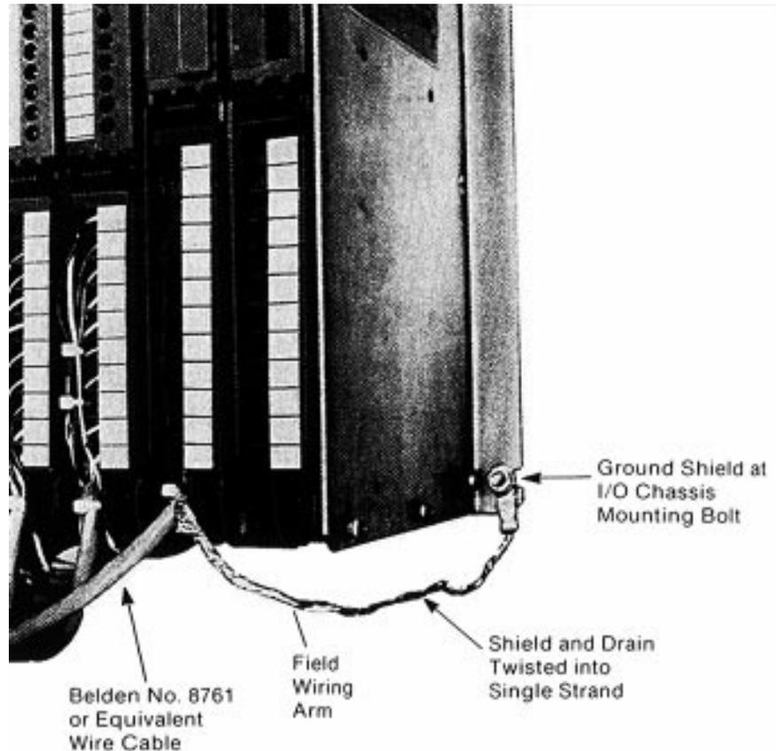
Because the module is extremely sensitive to the analog signal, care should be taken to prevent noise and interference from destroying the integrity of the signal. For detailed installation instructions, refer to publication 1771-803, Analog Input Systems User's Manual.
