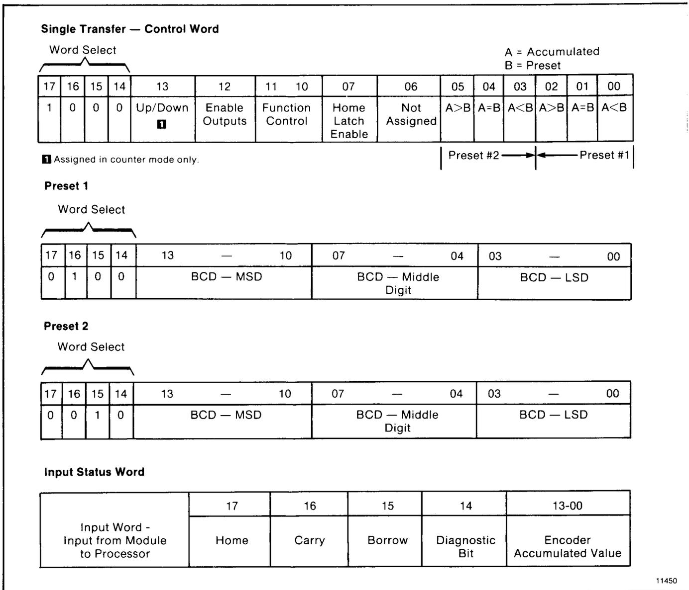
Since block transfer moves words of data simultaneously, rather than one at a time, there is no need to label which word of data is being transferred. Therefore, it is not necessary to distinguish the control word and each of the preset words (figure 7).
