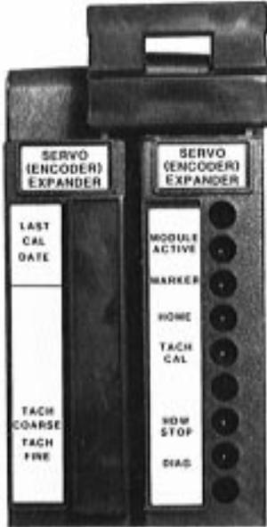
The 1771-ES expander has six indicators. With the PC processor in the run mode, the indicators have the following functions:
