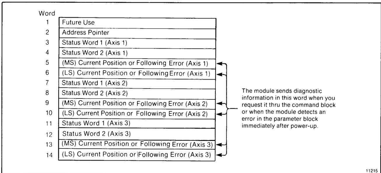
The first block transfer after power-up writes a 6-word status block into the data table. After that, the status block consists of 6 words for a 1-axis system, 10 words for a 2-axis system, or 14 words for a 3-axis system. You establish the address of the status block thru the block transfer read instruction. Because axis command and status data is stored in the data table, axis motion control can be interactive with other axes, discrete I/O, and report generation.
