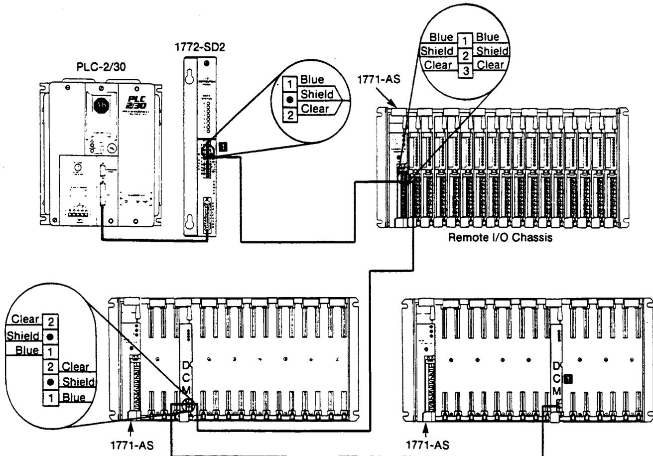
**1** Terminator Resistor: 150ohm, 1/2watt
