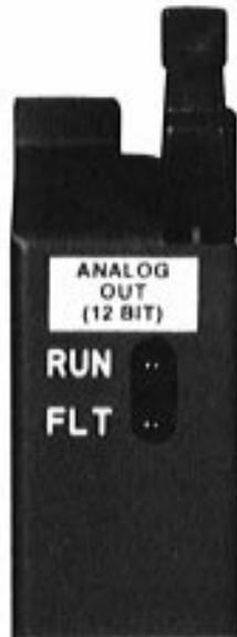
If a self-test fault occurs, the Input Image Table word of the programmable controller which corresponds to the location (address) of the module indicates the diagnostic code 00000000 (00 hex). The write block transfer is also inhibited. The outputs will stay at their present state because writing to the digital to analog converter will result in unpredictable signals sent to the outputs.
