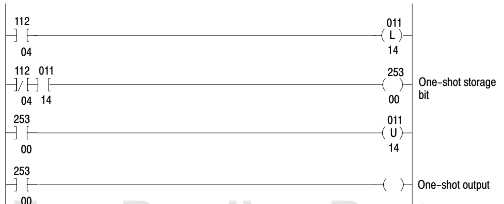
Figure 11.5 Trailing Edge One-Shot
