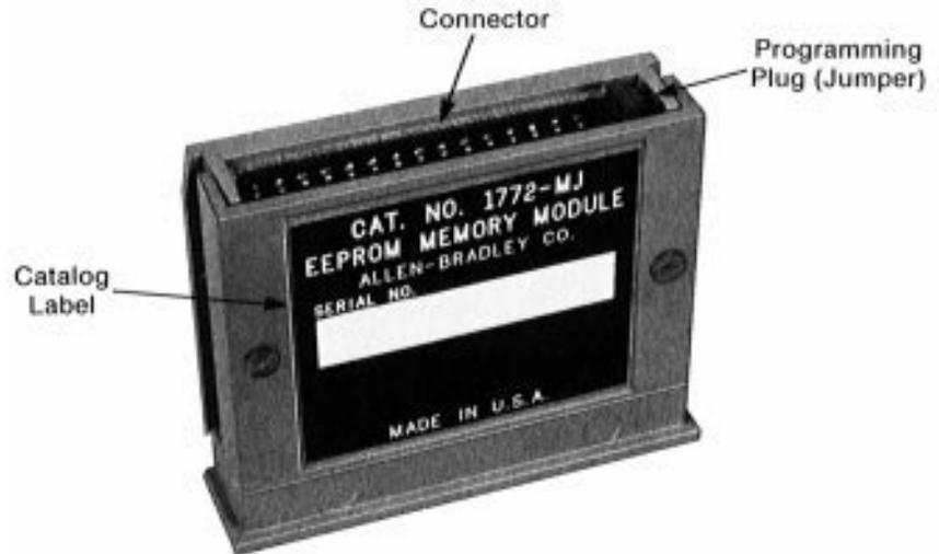
You can duplicate and transfer processor memory from CMOS RAM to the EEPROM module when the processor is in remote program mode. You can select one of the following three modes that the processor will use to establish its memory when recovering from a power loss. The processor transfers back-up EEPROM automatically to its CMOS RAM, transfers only if its CMOS RAM is invalid, or does not transfer back-up EEPROM.
