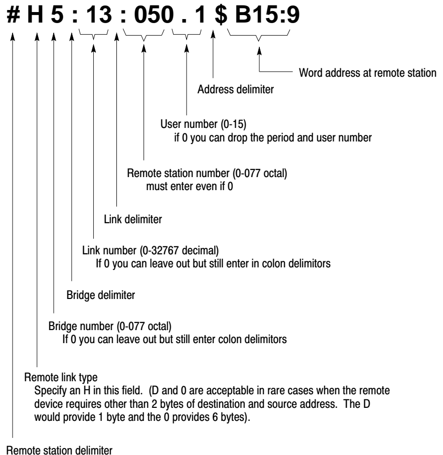
Figure 5.9 Example for Addressing a Remote Station Located on a Remote DH+ Link
