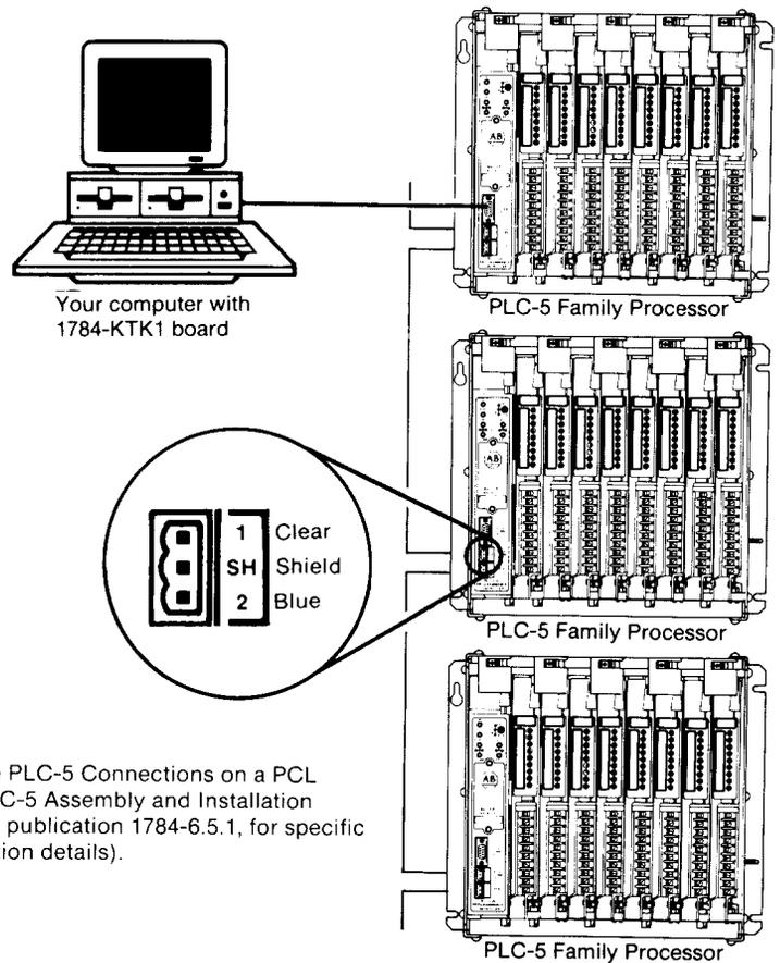
Multiple PLC-5 Connections on a PCL
