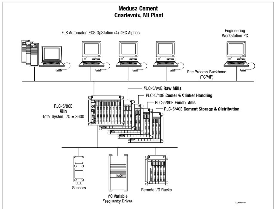
controlling and/or monitoring the performance of variable frequency drives as well as an on-line X-ray system that adjusts the raw mix feeders based on a compositional analysis.
