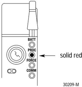
In some instances, typically larger configurations, when the processor attempts to configure the network (either after a processor download or after a channel 2 configuration edit), the processor may determine that the ControlNet configuration exceeds the processor bandwidth. It will then display a major fault with the processor RUN/FAULT status indicator solid red. This can occur prior to a 205 fault code being generated. If this occurs:
