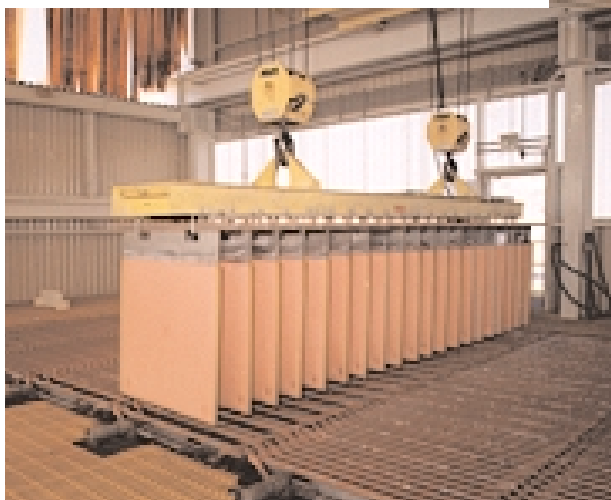
An Allen-Bradley PLC-5 programmable controller and 1771 N-Series I/O continuously regulates copper concentration during the electrowinning process (left), while another PLC-5 controller and a PanelView display provide control of a cathode stripping machine (above).
