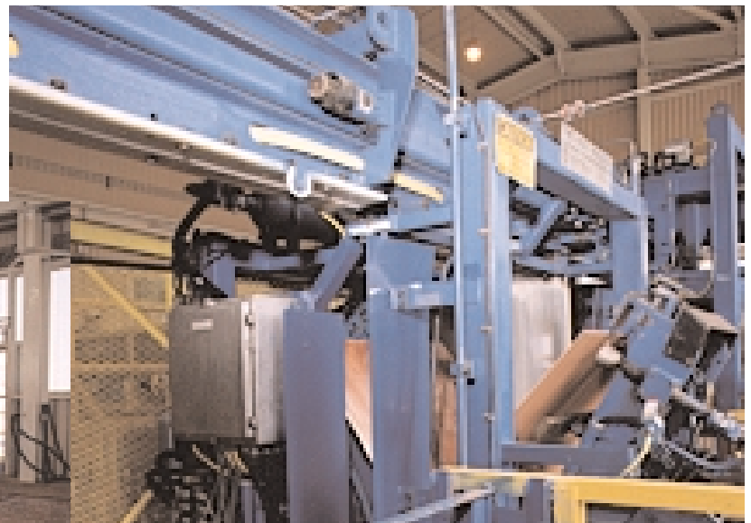
An Allen-Bradley PLC-5 programmable controller and 1771 N-Series I/O continuously regulates copper concentration during the electrowinning process (left), while another PLC-5 controller and a PanelView display provide control of a cathode stripping machine (above).
