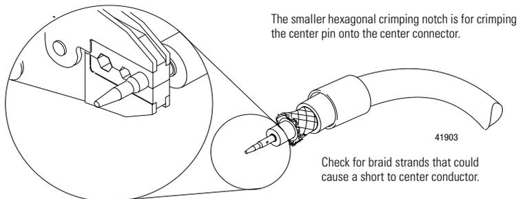
8. Slide the ControlNet connector onto the cable. Push the connector body on tight until the center pin tip is flush with the inner ground ring.
