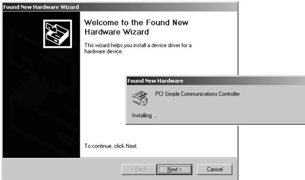
Windows 2000 identifies the 1784-PM02AE card as a PCI Simple Communications Controller.
