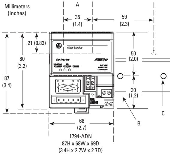
A = Mounting hole dimensions for optional mounting kit
