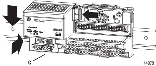
When the adapter is locked onto the DIN rail, gently push the flexbus connector into the adapter to complete the backplane
