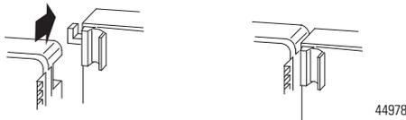
7. Complete the adapter mounting as shown below. Push down and in at the same time to lock the adapter to the DIN rail. If the adapter does not lock in place, use a screwdriver or similar device to move the locking tab down while pressing the adapter flush onto the DIN rail, and release the locking tab to lock the adapter module in place. If necessary, push up on the locking tab to lock.
