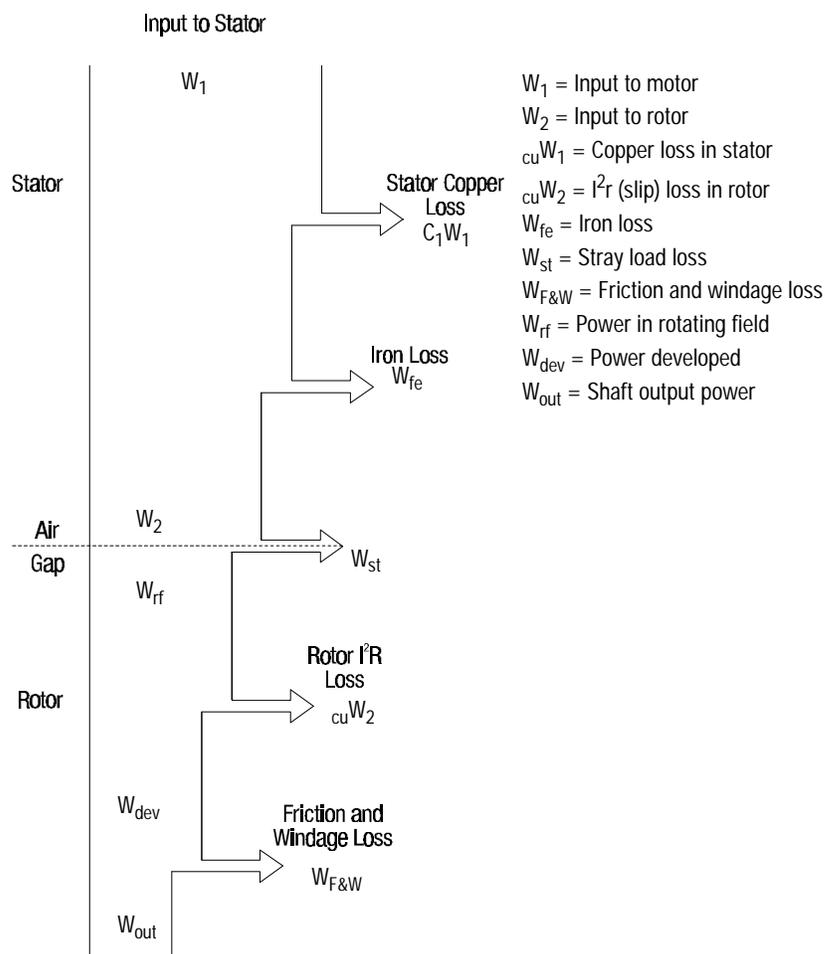
During normal running conditions, the current flowing through the stator windings produces stator copper losses proportional to the square of the current ( $I^2$ ). However, the losses in the stator iron are due to magnetization and eddy currents, which are a function of voltage.
