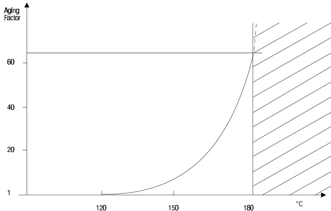
Short-time over-temperatures do not reduce motor life considerably as long as certain limits are not exceeded. Motor manufacturers intentionally permit such short-time over temperatures during the start-up period. This can also be done for normal motor operation, i.e., a motor can be selected according to the desired time of service rather than to keep within the rated values of load.
