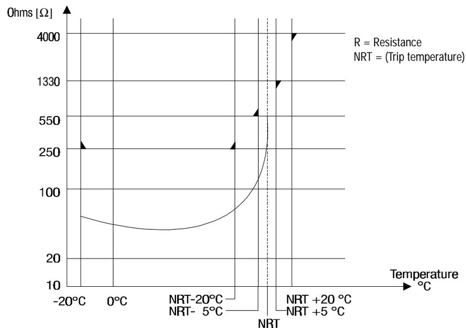
The trip or release temperature is determined by the sensor that is selected. So, the protective device cannot change the trip point. The motor manufacturer selects the sensor set to the correct detection temperature to match the insulation class of the motor windings. These sensors are embedded into the windings when the motor is built. If a warning function is required, a separate set of sensors having a lower response temperature is required.
