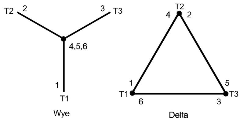
Typical Wye-Delta starters are made up of magnetic contactors that switch from the Wye to Delta connections, and a timing unit that controls the switching. When the operator presses the start button, the line and Wye contactors close and the motor starts. Full voltage is not
