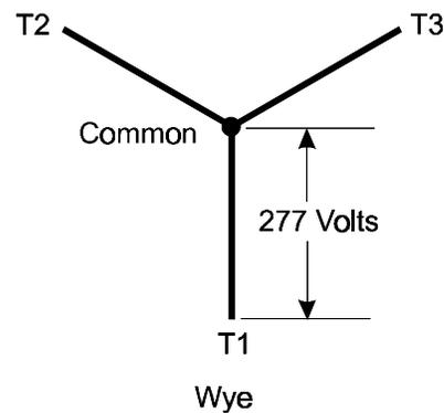
This connection reduces the voltage by the square root of three. For example:
