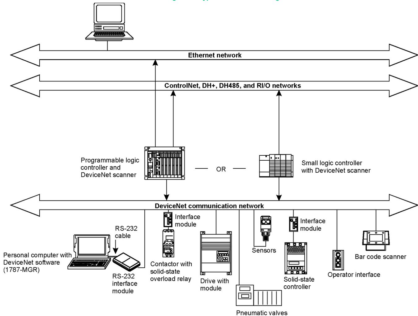
Other benefits of networks like DeviceNet is the significant reduction in installation and wiring costs. Traditionally, systems have typically required a large number of wires and a central control system to perform such tasks as reading the switches and driving the motor to perform the desired action. The large number of wires used for control not only increases development time, but also increases the risk of malfunctions.
