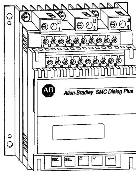
Many solid-state controllers offer the choice of four starting modes: soft start, current limit start, dual ramp start, or full voltage start in the same device. You can select the starting mode of the solid state controller and adjust the soft start ramp time, as well as the current limit maximum value, which enables selection of the starting characteristic to meet the application.
