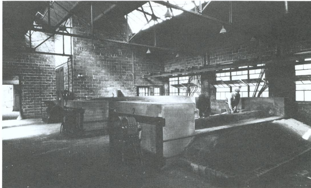
One of the steps in the early days of the manufacture of compression resistor tubes was to fire the discs beneath a mound of electrically heated dirt. Furnaces are now used for this purpose. The discs have continued to be made in the same department, the Powder House, which is in this same location today.
