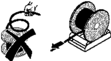
**Figure 3 Use a Device to Uncoil Fiber Optic Cable**
