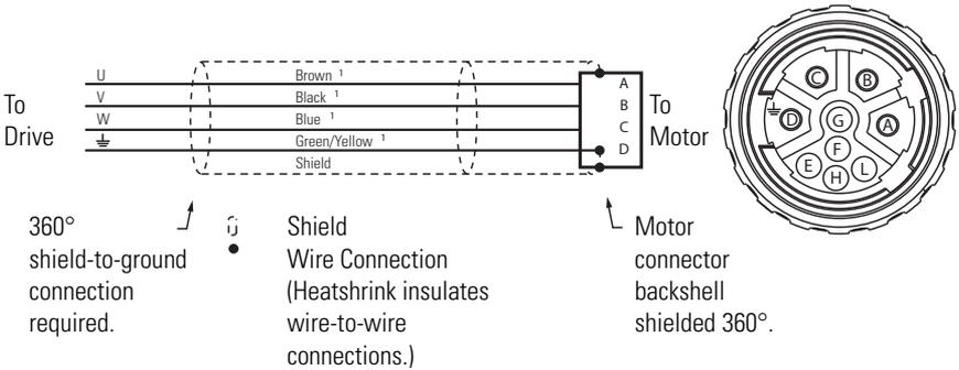
1 Wire gauge (10, 12, 14, or 16 AWG) and connector keying varies based on motor and power requirements. Refer to Kinetix Motion Control Selection Guide, publication [GMC-SG001](#), for additional information.
