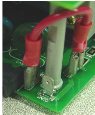
Ungrounded Configuration CON7 to CON6
