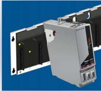
*The innovative Power Rail is just one of the many time-saving features of Kinetix 6000. The Power Rail's simple design allows you to mount an axis in less than a minute. It requires just five bolts to mount up to 8 axes, replacing as many as 32 bolts used by other systems. Modules easily attach by hooking to the top, rotating down onto the connector and securing one screw. With the Power Rail, installation time and related costs are significantly reduced.*
