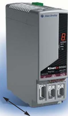
**Exceptional performance.** Advanced control capabilities provide greater precision and throughput, allowing you to meet demands for increased productivity. To help gain that added productivity, Kinetix 6000 offers an impressive velocity bandwidth greater than 400 Hz and a current loop bandwidth greater than 1300 Hz, double the performance of similar products.
