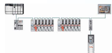
Linear Ethernet segments greatly extend the length of the application. There's no need to run cables from each device back to a centralized switch.
